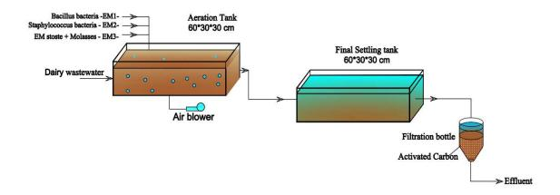
Figure 3. Scheme of the Experimental pilot.
