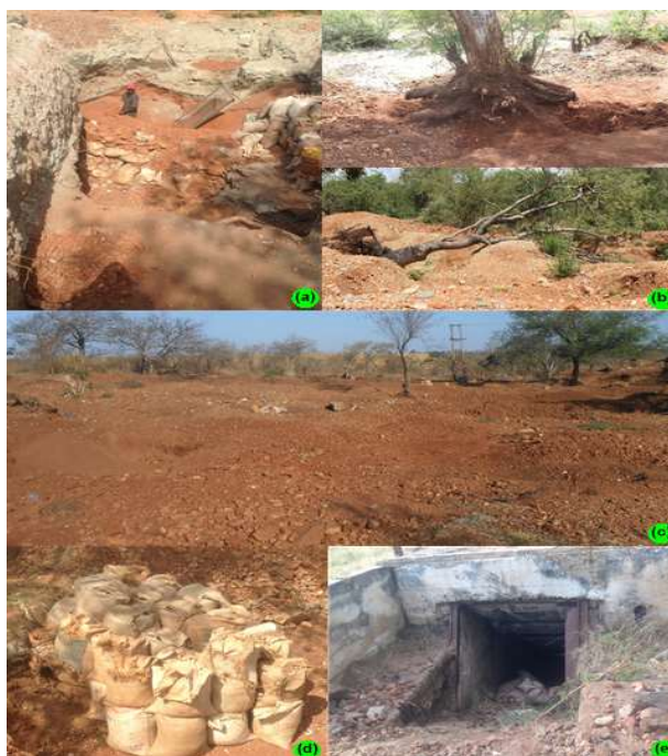
Figure 5. (a) is an illustration of artisanal gold mining activities (Mhlongo et al., 2019a), (b) show the effect of the mining process on trees, (c) show the scattered gravel waste on mined out areas, (d) is the bags of gold bearing sediments ready for transported to the clients, and (e) show the bags of material coming from underground through the inclined shafts.
