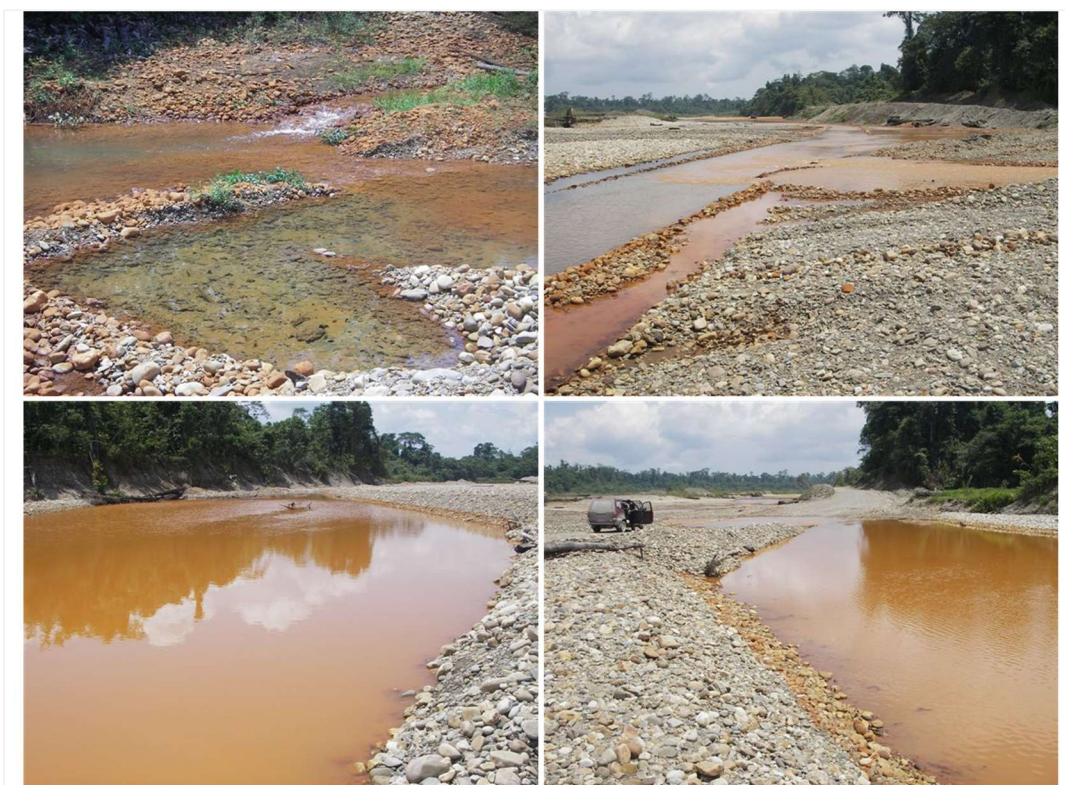
Figure 2. AMD seepage that passes the edge of the ModADA East embankment at MP 36 to Kopi river in 2007.
