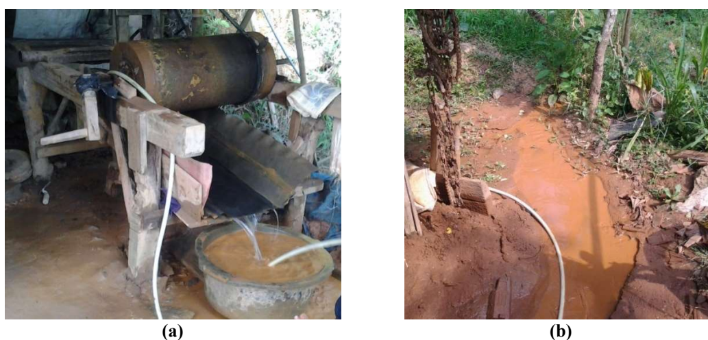
Figure 1. Slurry of amalgamation waste (a) and slurry spill on the soil surface (b).
