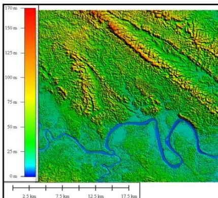
Figure 6. DEM ALOS PALSAR using interferometry. Area in Batang Hari, Jambi.
