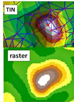
Figure 3. Example of TIN and DEM from terrestrial survey.
