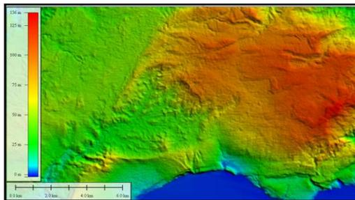
Figure 2. Example DTM integration from IFSAR-ALOS PALSAR-IceSAT/GLAS-SRTM C- X SAR. Area in Rote Islands.
