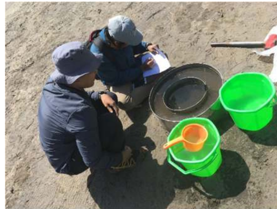
Figure 8. Soil infiltration was measured using a double-ring infiltrometer following the falling head method.
