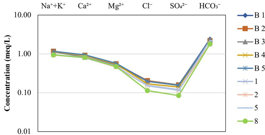
Figure 5. Schoeller diagram of reservoir water samples with water at leakage points 1, 2, 5, and 8.
