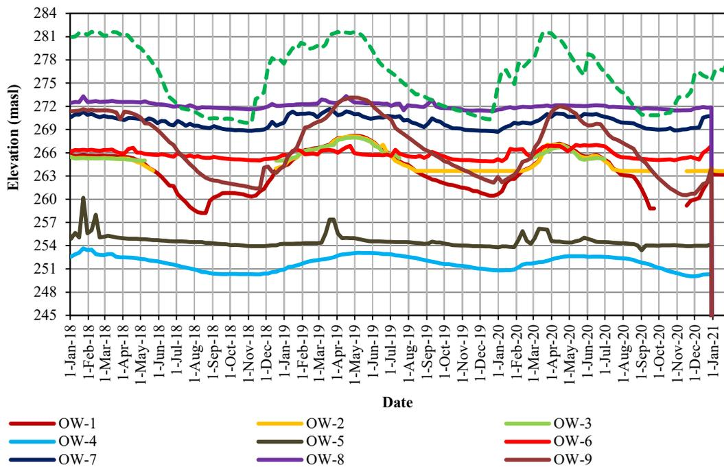
Figure 3. Patterns of fluctuations in reservoir water level and groundwater level.
