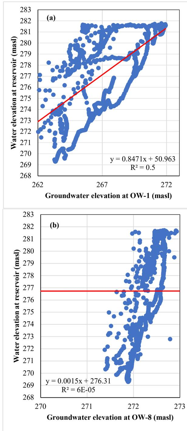
Figure 4. Comparison graph of reservoir water elevation with groundwater level OW-1 (a) and OW-8 (b).
