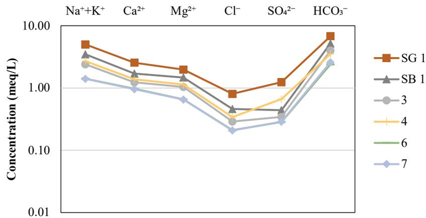
Figure 6. Schoeller diagram of water samples SG1 and SB1 with water at leakage points 3, 4, 6 and 7.
