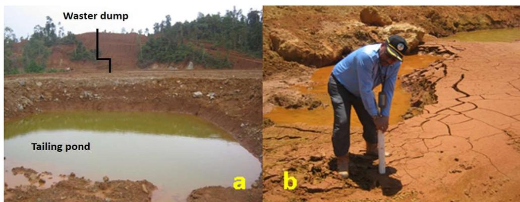
Figure 2. (a) Tailing dams, (b) Sample collecting process in tailing sediment.
