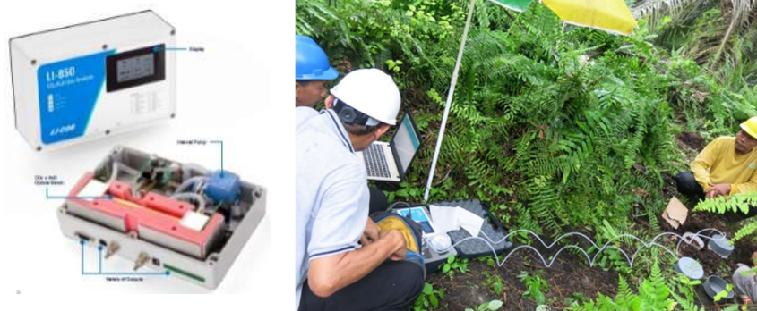
Figure 3. Measurement of CO_2 flux at the study site using a portable LI-COR 830 Gas Analyzer.
