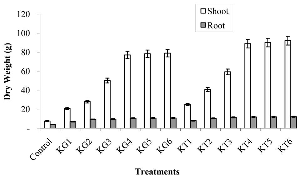
Figure 2. Effects of application of *Gliricidia* and *Tithonia* prunings on maize shoot and root dry weights (KG: *Gliricidia* pruning; KT: *Tithonia* pruning; 1, 2, 3, 4, 5 and 6 are rates of 5, 7.5, 10, 20, 40 and 80 t/ha, respectively).
